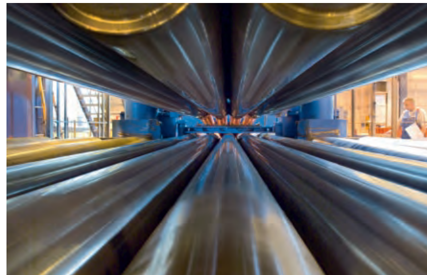
Danieli Multi-Cassette leveler at Anshan Iron & Steel
