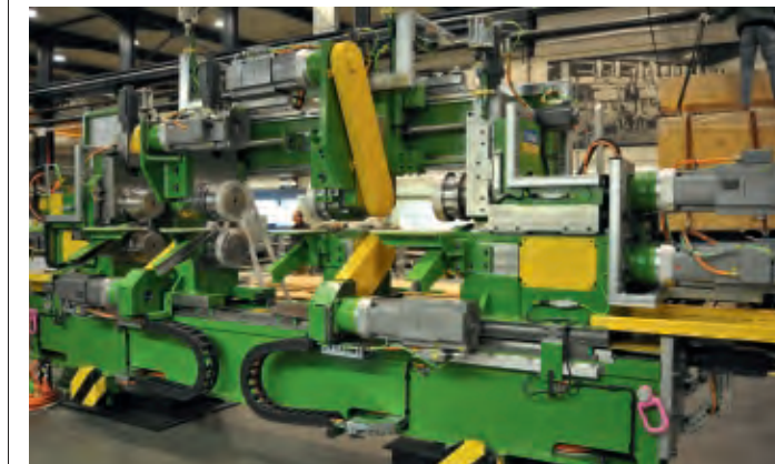
Assembly of a high-tech CNC slitting shear in Danieli Fröhling's workshop in Meinerzhagen, Germany.
