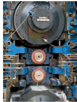
Detail of a four-high high-tech cold mill stand.
