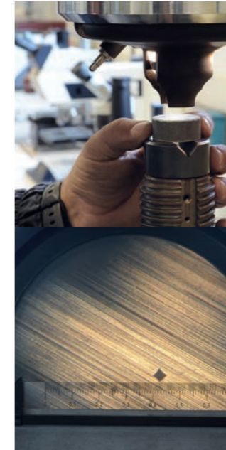
Hardness tests being carried out on the seal end plate after the Nitreg process.
