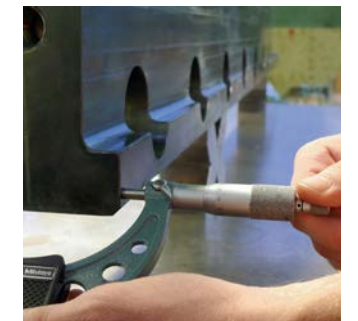
Dimensional check of DanCut 710 blades after precipitation hardening treatment.
